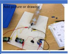
3 wires, 1 lightbulb , 2 battery and 1 homemade switch
