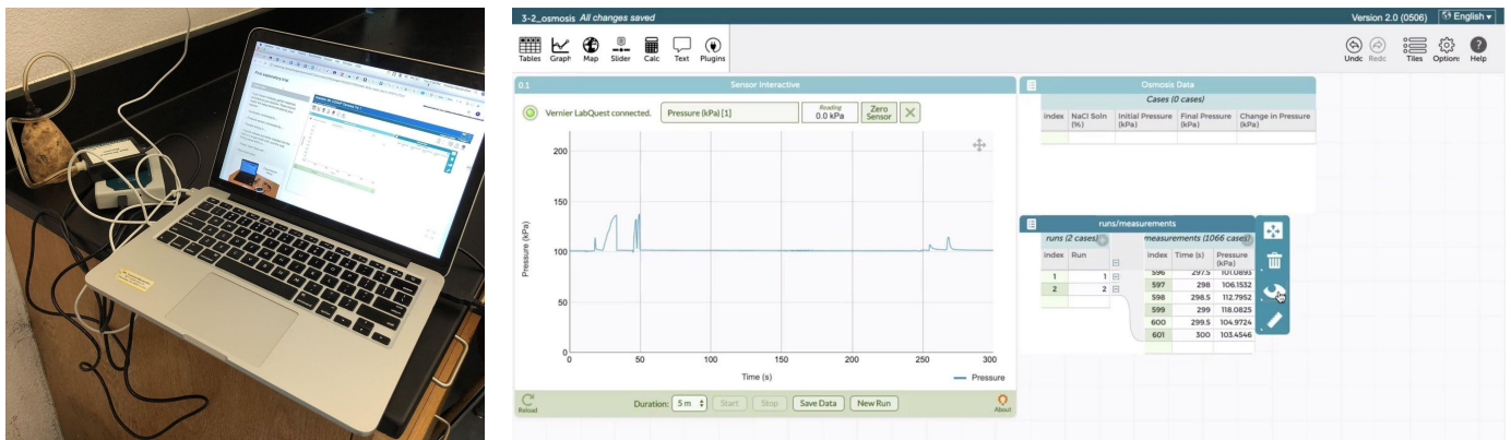
Figure 1. The potato osmosis lab setup. A potato with a pressure sensor attaches to the laptop (left). Data was displayed in real time on the computer screen as students produced data from the pressure sensor, which was then exported into the data analysis software (right). These students have not rescaled their graph and so the signal appears as a horizontal line; the slope is not visible.
