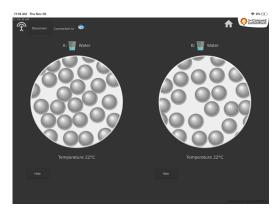
The Thermoscope screen shows the emoji of the Thermoscope that is connected. The sliders are replaced by the temperature readings of the probes. The motion of the particles reflects the temperature measured by the probes.
