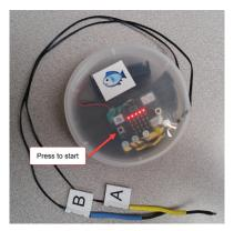
Turn on your Thermoscope probes by pressing down on the flexible cover close to the smaller emoji symbol inside the container. Five lights in a row show that the Thermoscope is ready to be connected.
