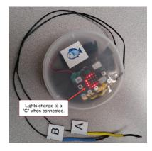
The lights on the Thermoscope probes will change to a "C" for connected.
